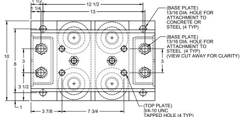
RATED **SPRING RATE** RATED SEISMIC MOUNT DEFLECTION **COLOR CODE** LOAD (LBS) (LBS/IN) (IN) M4SH-2E-4000 4000 2.00 2000 TAN M4SH-2E-5600 5600 1.87 3000 RED 2.13 M4SH-2E-6400N 6400 3000 TAN/ RED 1.71 M4SH-2E-7200 7200 4210 DK GRAY M4SH-2E-8200 8200 1.64 5000 DK BLUE 9000 1.62 5556 DK BLUE/BLACK M4SH-2E-9000N1 9840 1.64 6000 DK BLUE/RED M4SH-2E-9840N M4SH-2E-10800N 10800 1.64 6600 DK BLUE/DK GREEN
